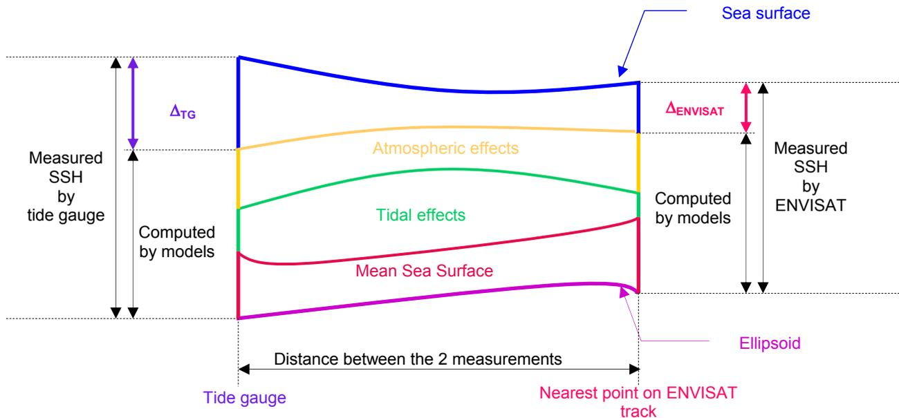
**Figure 2: Determination of the RA-2 bias compared with in situ tide gauge measurement.**
